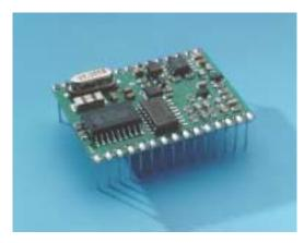
in-line printed circuit board. The Series 2000 Micro Reader is equipped with a serial communication interface and works together with a 47  $\mu$ H low-Q antenna that eliminates the need to tune the system to resonance.
